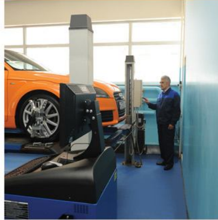
Techno Vector 6 is designed to check and perform wheel alignment on vehicles with 12 to 24" disks
